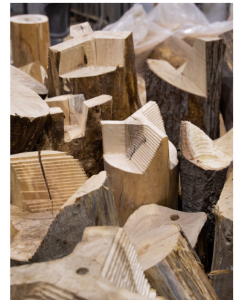
Figure 3. LOG KNOT plan and section. View of robotically CNC milled tri-part mortise and tenon joinery studies. Image and drawing by Cornell RCL.
